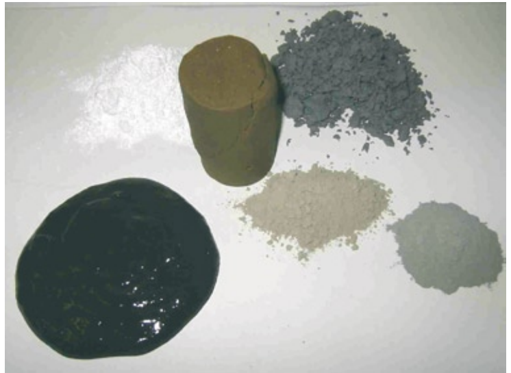
Picture: Materials from laboratory testing: dredged sediment, cement and fly ash; gypsum, stabilised specimen and fibre clay (paper industry by-product)
